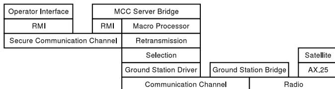
Fig. 8. Protocol stack for communication with the satellite.
