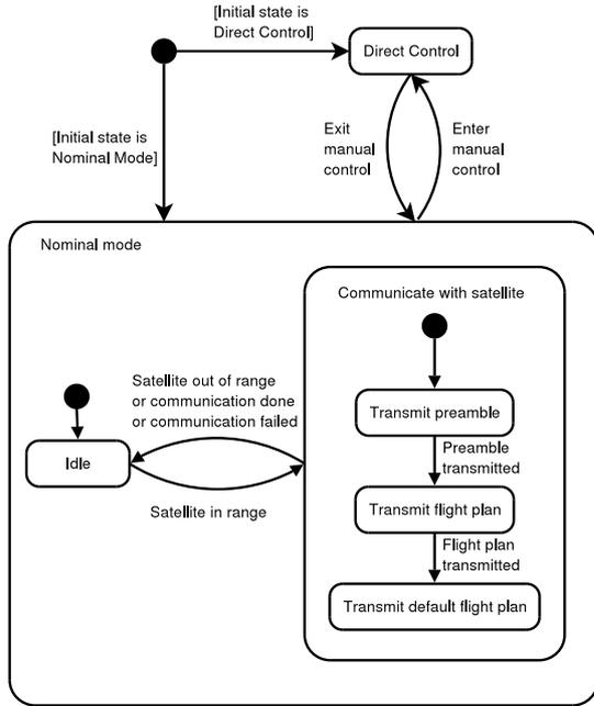
Fig. 6. State diagram of overall states.
