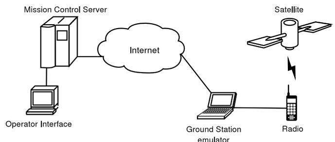
Fig. 12. Communication path for the second preliminary test.
