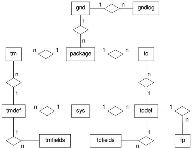
Fig. 7. ER-diagram for the database without attribute definitions.
