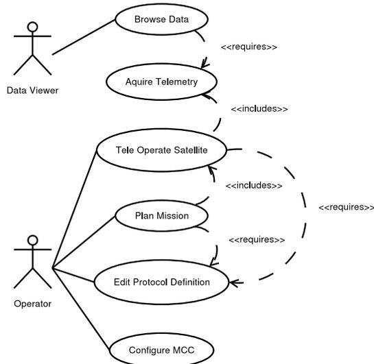
Fig. 1. Use case diagram for the MCC.
